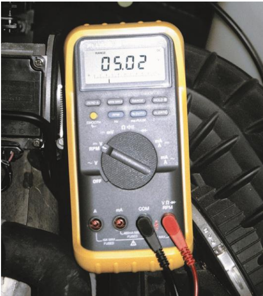
Figure 8. Measuring the reference voltage at a throttle position (TP) sensor.
