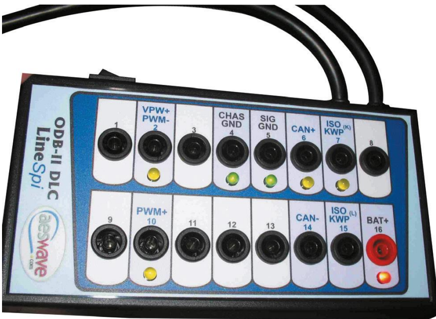
Figure 15. This breakout box is equipped with LEDs that light when data circuits are active.
