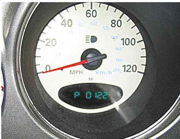
Figure 5. DTC P0122 indicates a Throttle/Pedal Position Sensor/Switch "A" Circuit Low Input.
