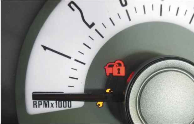
Figure 12. A security system fault will cause the warning lamp to flash and may cause a no-start.
