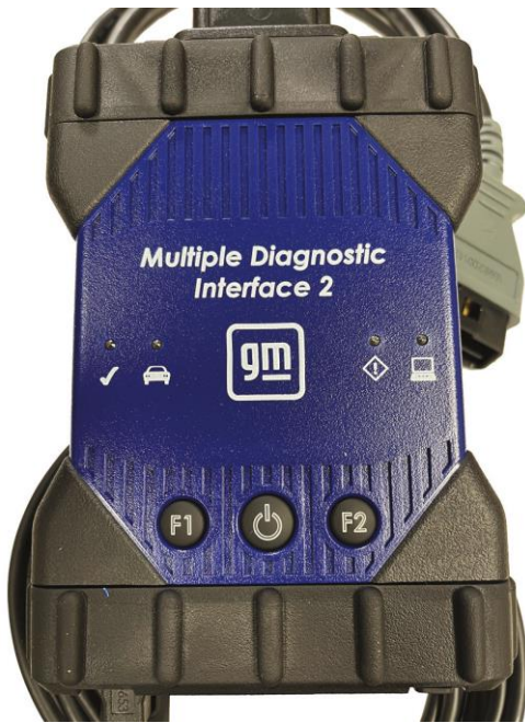
Figure 2. The GM MDI2 connects between the DLC and a dedicated laptop computer to make up the complete scan tool.
