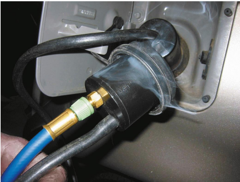
Figure 13. Smoke testing shows that the gas cap seal is leaking.
