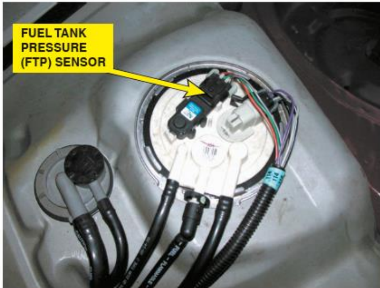
Figure 14. The FTP sensor is often part of the fuel pump module.
