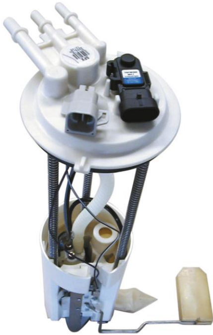
Figure 10. A typical fuel-pump module assembly, which includes the pickup strainer and fuel pumps, as well as the fuel pressure sensor and fuel level sensing unit.
