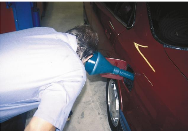
Figure 12. Listening to confirm pump operation.
