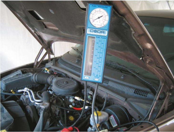
Figure 16. A tester that measures both pressure and volume.
