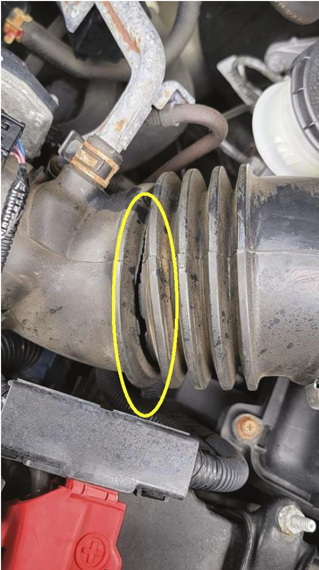
Figure 21. Inspect ducting for cracks and splits.
