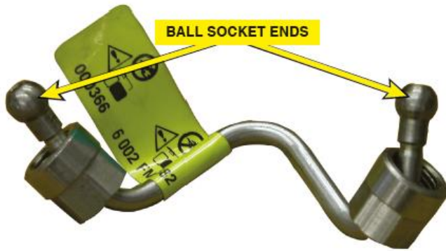
Figure 19. A GDI high pressure line.
