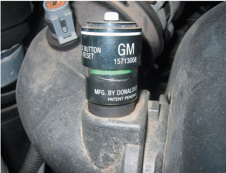
Figure 21. An air filter restriction indicator turns red when it detects enough restriction to require a filter replacement.
