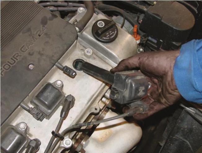
Figure 5. Check the COP coil for arcing or corrosion.
