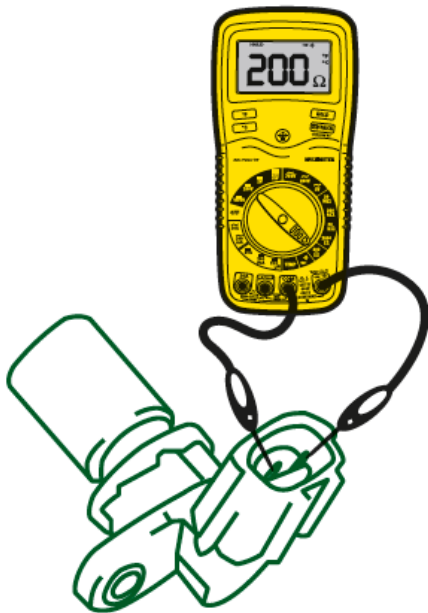
Figure 12. Checking CKP sensor resistance.
