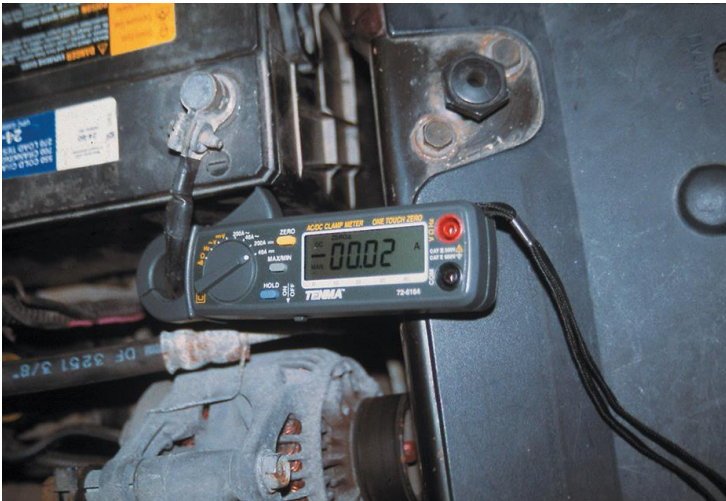
Figure 19. An inductive clamp-on meter can measure parasitic drain.
