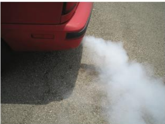
Figure 2. Excessive white exhaust indicates water or coolant in the combustion chamber.
