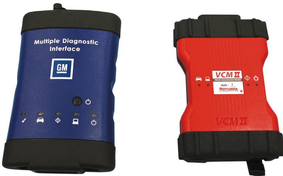
Figure 29. Tools required for module reprogramming.
