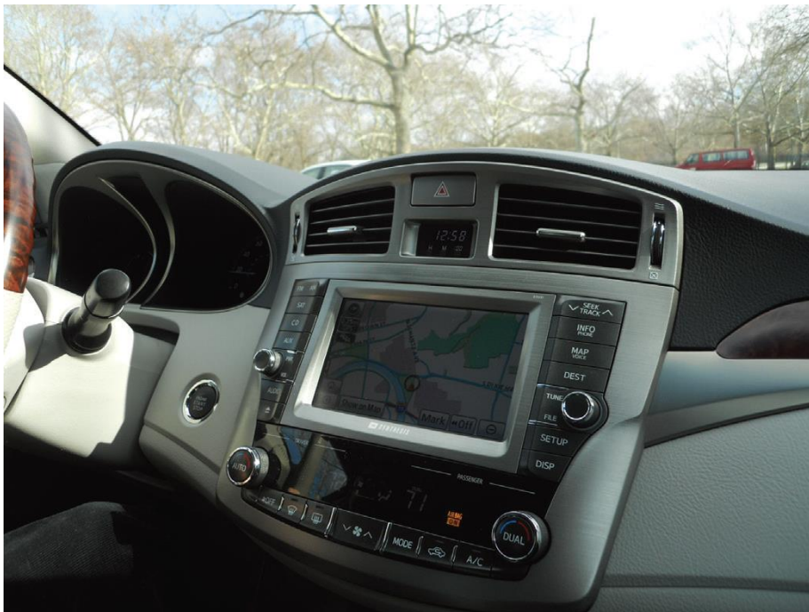
Figure 16. A navigation system with the HVAC controls below.
