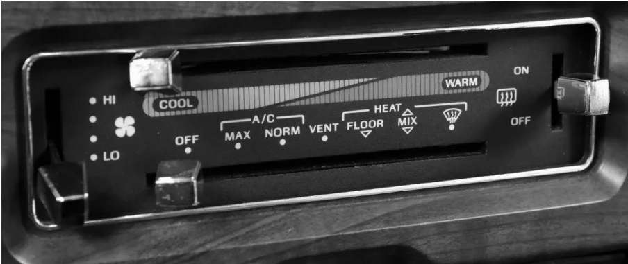
Figure 18. Cable-operated temperature and mode controls.
