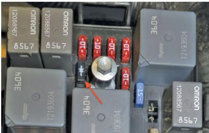
Figure 12. A/C compressor clutch spike suppression diode.
