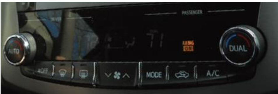
Figure 28. HVAC operator input panel (control panel).
