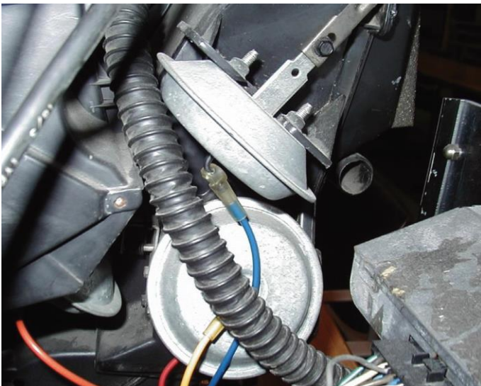
Figure 4. Many older vehicles used vacuum actuators to move the HVAC doors.
