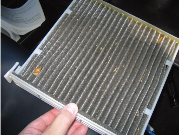
Figure 30. A dirty cabin filter will reduce evaporator airflow.
