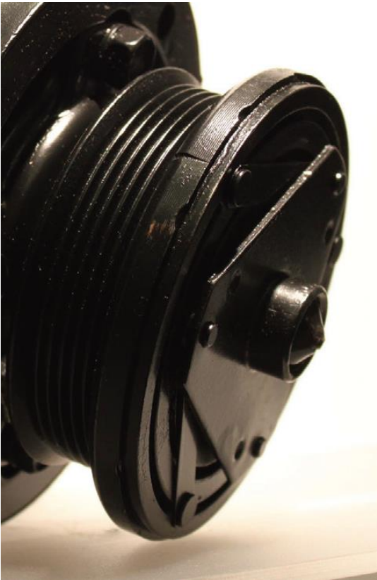
Figure 14. An electromagnetic compressor clutch.
