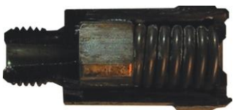
Figure 36. A high-pressure relief valve contains a strong spring that keeps the valve closed unless high-side pressure (from the left) forces it open.
