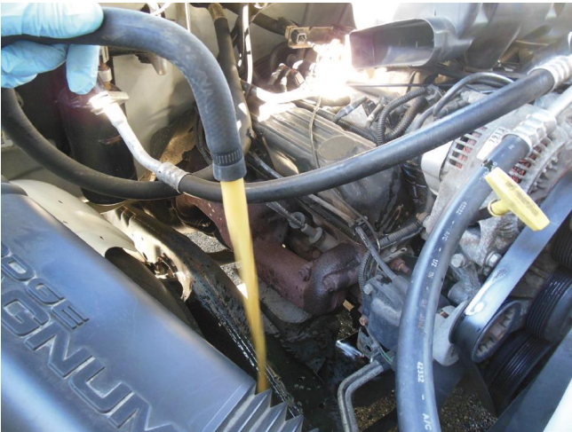
Figure 45. Flushing the heater core.
