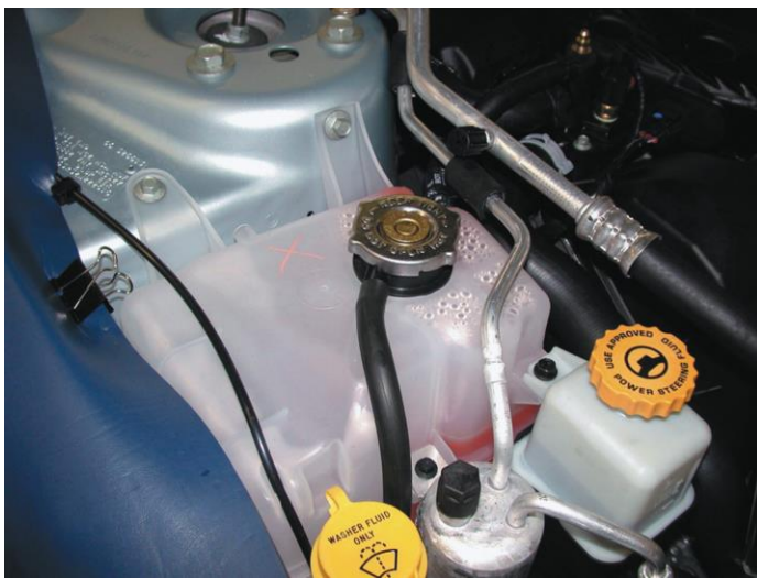
Figure 35. Surge tank and pressure cap.
