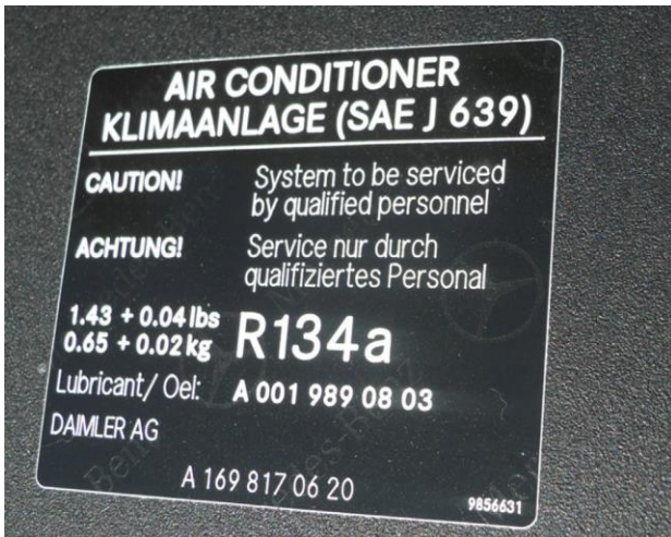
Figure 17. This vehicle specifies R-134a refrigerant.
