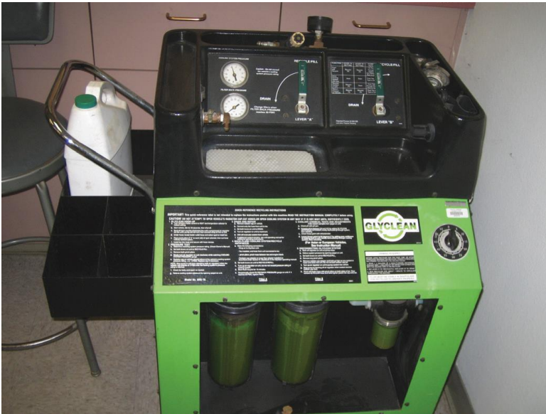
Figure 40. A coolant exchange machine takes care of flushing and refilling the cooling system.
