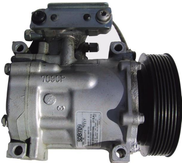
Figure 5. The compressor is mounted to the engine and driven by a belt.
