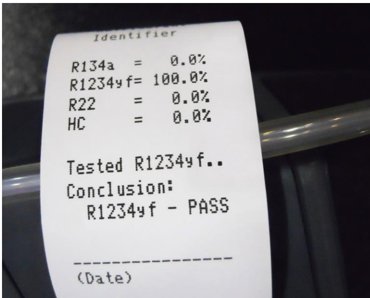
Figure 18. Identifier printout shows 100% R-1234yf.
