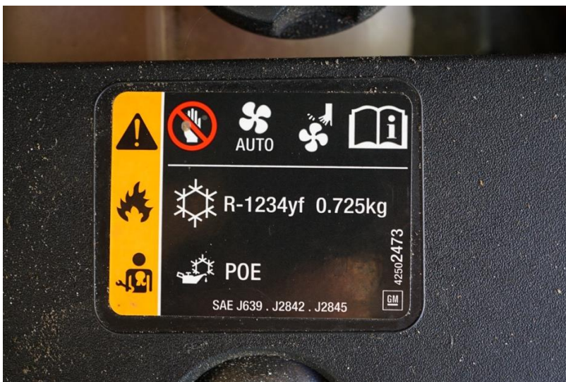
Figure 21. This vehicle uses R-1234yf refrigerant and POE oil.
