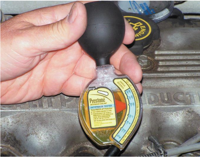
Figure 30. Checking the freezing temperature of the coolant using a hydrometer.
