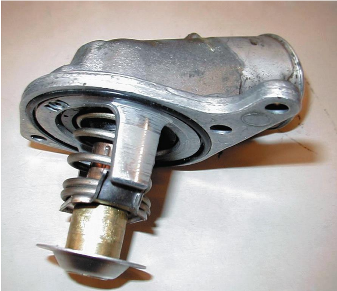
Figure 39. This thermostat seals with an O-ring instead of a gasket.
