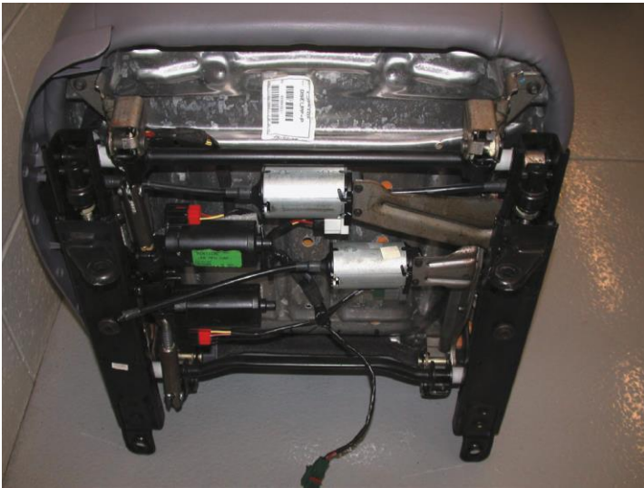
Figure 2. A power seat uses electric motors under the seat, which drive cables that extend to operate screw jacks (up and down) or gears to move the seat forward and back.
