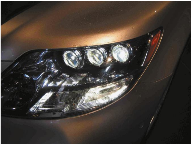
Figure 5. LED headlights usually require multiple units to provide the needed light.
