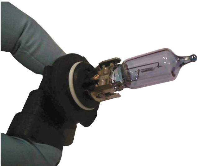
Figure 11. Handle a halogen bulb by the base to prevent the skin's oil from getting on the glass.
