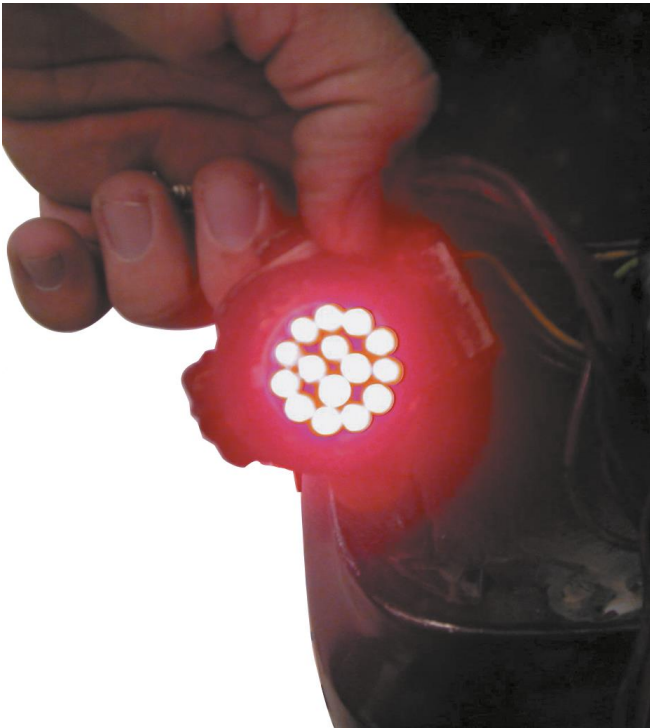
Figure 10. A replacement LED taillight bulb is constructed of many small, individual light-emitting diodes.
