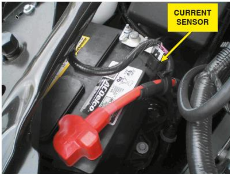
Figure 5. A Hall-effect current sensor attached to the positive battery cable is used as part of the EPM system.
