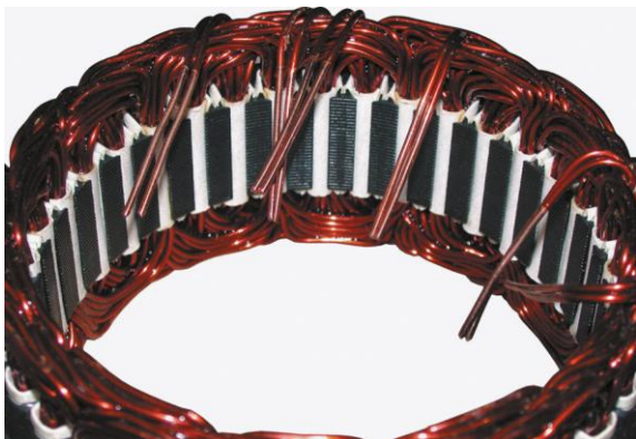
Figure 3. The stator has from three to six separate windings.
