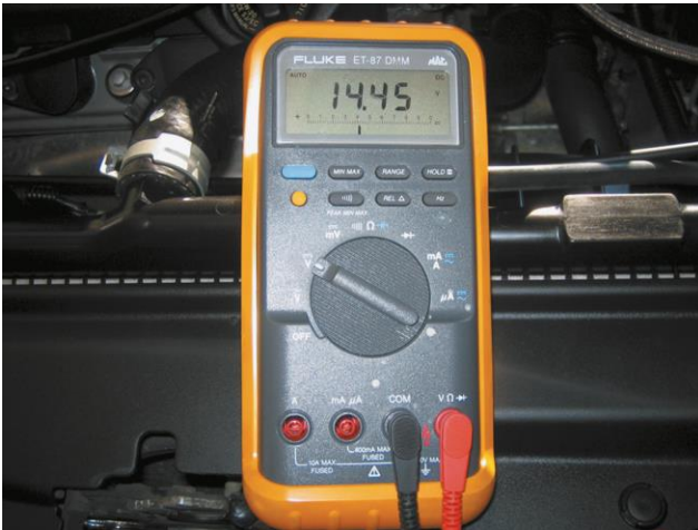
Figure 8. Charging system voltage test.
