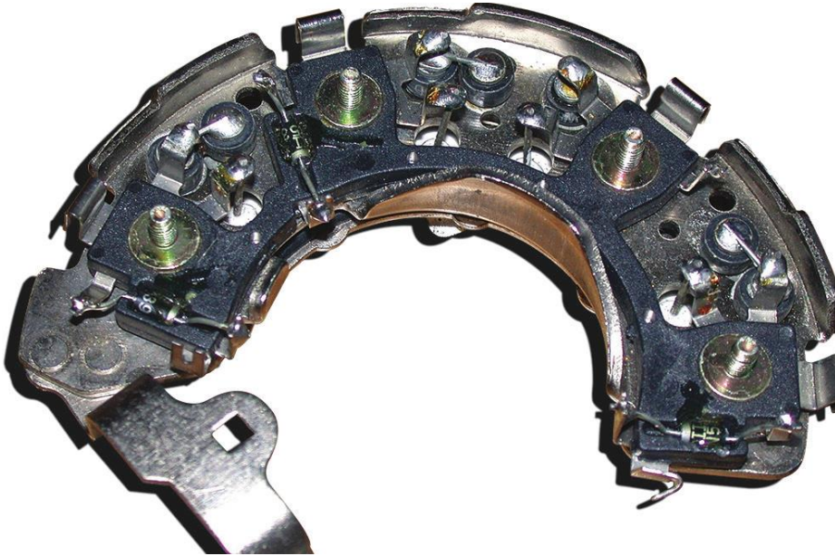
Figure 4. A rectifier bridge includes the diodes and heat sink for cooling.
