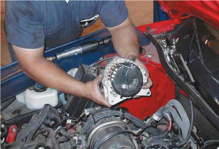
Figure 14. Alternator removal. Many alternators are difficult to access and will require the removal of other components.
