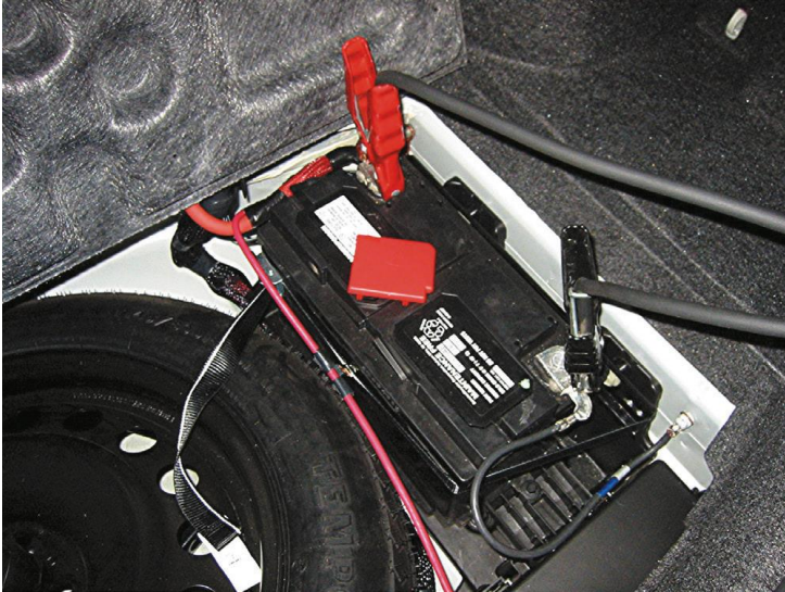
Figure 5. An AGM battery under the floor next to the spare tire in a hybrid-electric vehicle. A vent tube is used to route battery fumes to the outside of the vehicle.
