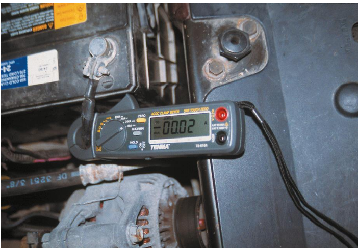
Figure 20. A mini clamp-on digital multimeter can be used to measure the amount of battery electrical drain that is present. In this case, a reading of 20 milliamperes (displayed on the meter as 00.02 ampere) is within the normal range of 20 to 30 milliamperes.
