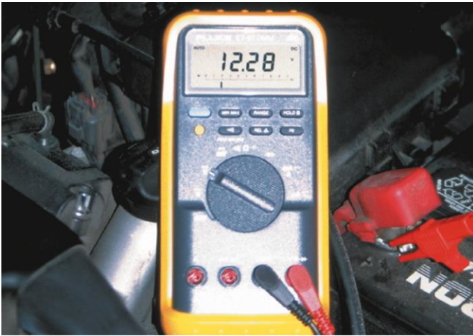
Figure 11. Measuring battery voltage.
