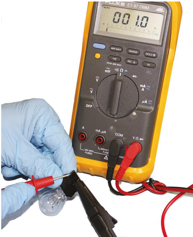
Figure 14. Using a digital multimeter set to read ohms ( \Omega ) to test this lightbulb. The meter reads the resistance of the filament.
