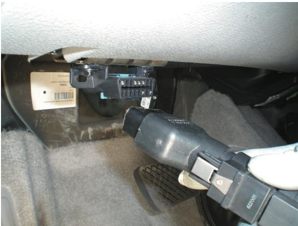
Figure 7. Connect a factory or enhanced scan tool to the data link connector (DLC) located under the dash on this vehicle.
