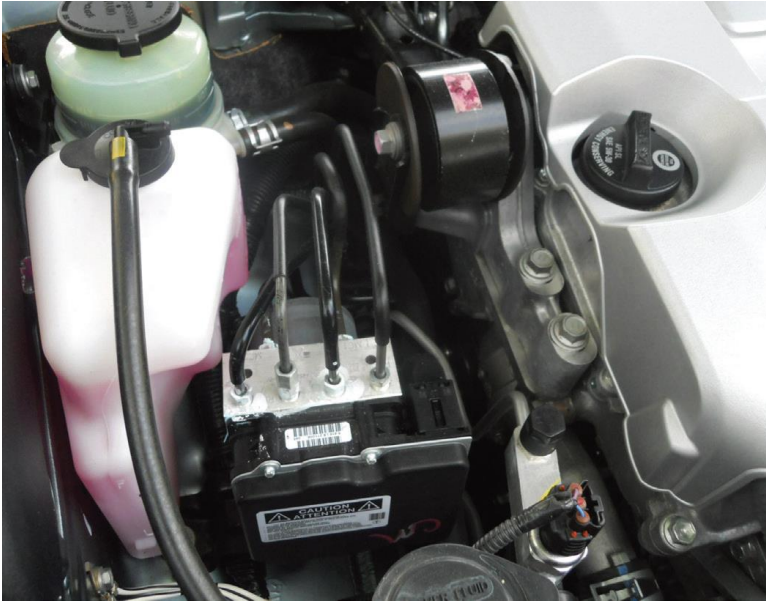
Figure 3. A four-channel ABS hydraulic modulator and EBCM.
