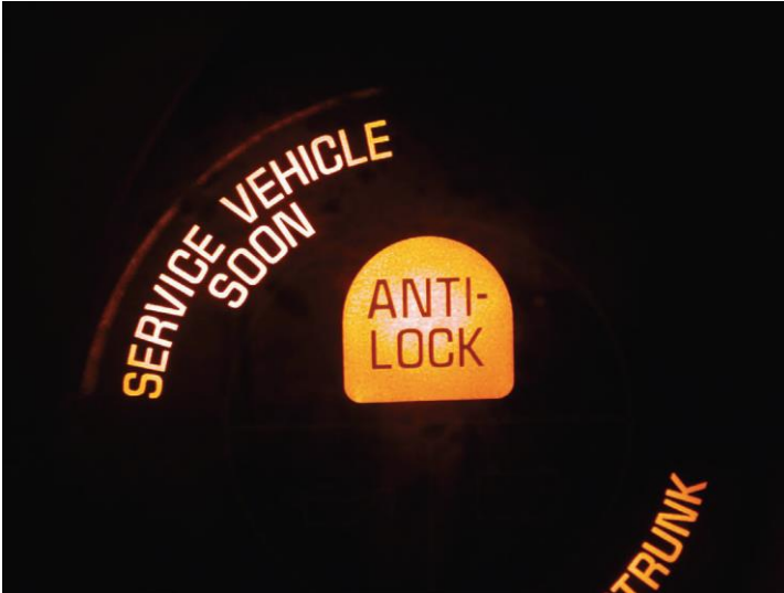
Figure 5. The amber ABS warning lamp comes on at start-up and stays on if there is a fault in the ABS.
