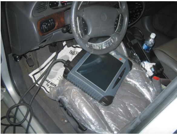
Figure 17. The use of a factory scan tool is often needed to diagnose the ESC system.
