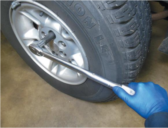
Figure 29. A torque wrench being used to tighten lug nuts on a pickup truck.
