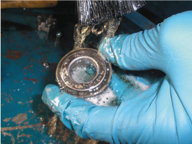
Figure 30. Cleaning the wheel bearing.
