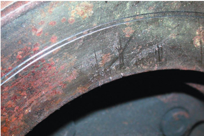
Figure 24. Scratch cuts are side-by-side. OK to proceed with machining.
