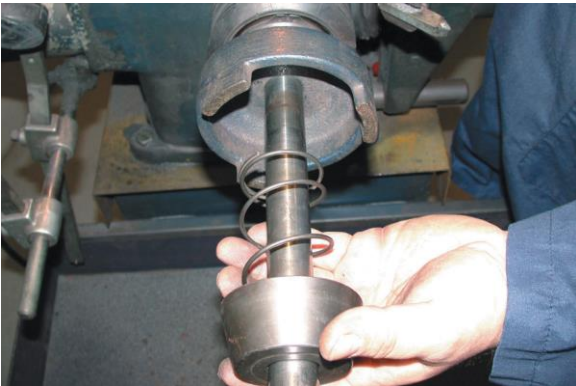
Figure 23. Use the correct cone and adapters to mount the rotor.
