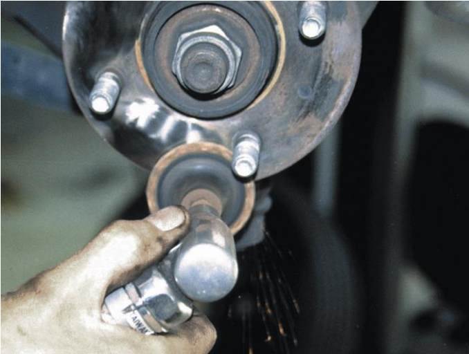
Figure 22. Cleaning the hub flange.
