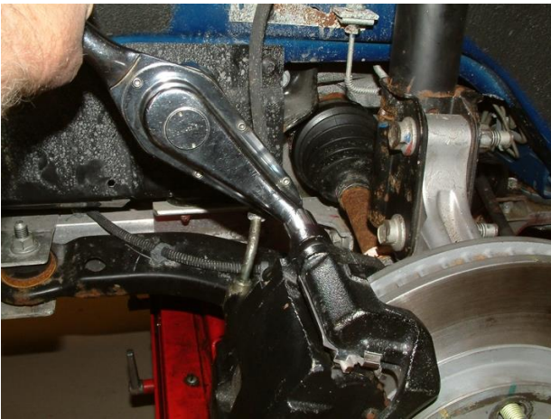
Figure 28. Tighten the mounting bolts to the proper torque.
