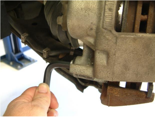
Figure 10. Loosen and remove the mounting bolts.
