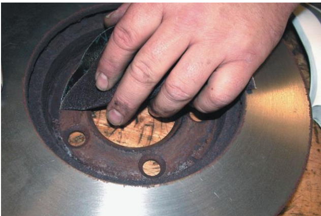
Figure 21. Cleaning the inside of the rotor.
