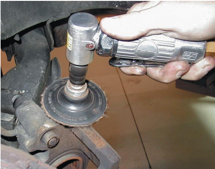
Figure 14. Cleaning the caliper mounting surface.
