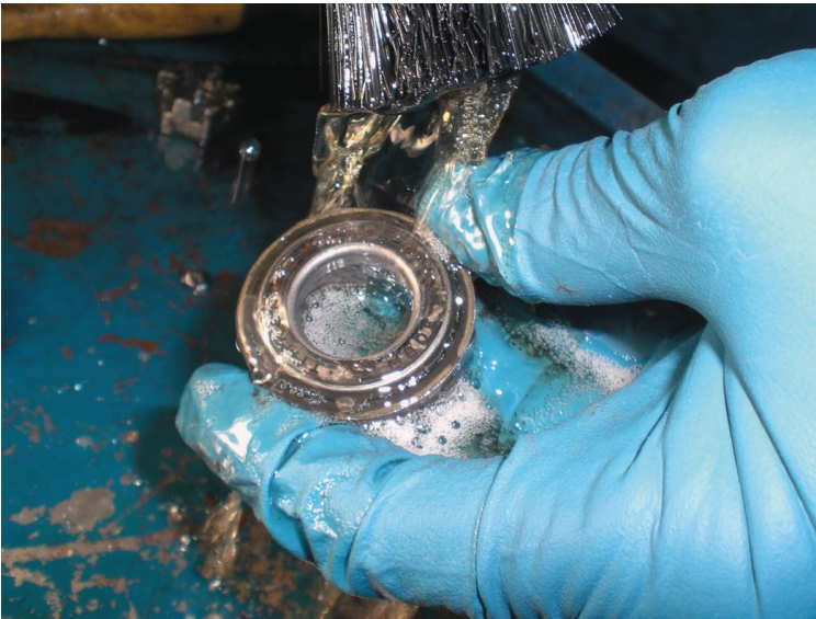
Figure 28. Cleaning the wheel bearing.
