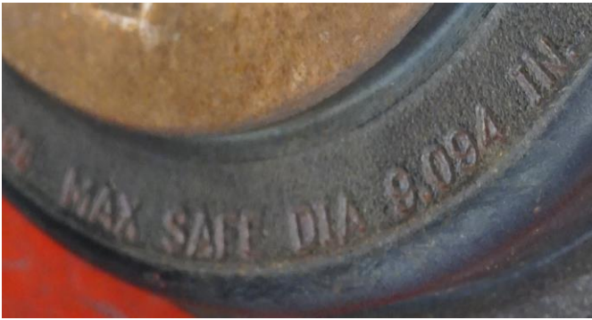
Figure 12. This drum can be machined to a maximum diameter of 9.064 in., leaving 0.030 in. for wear.
