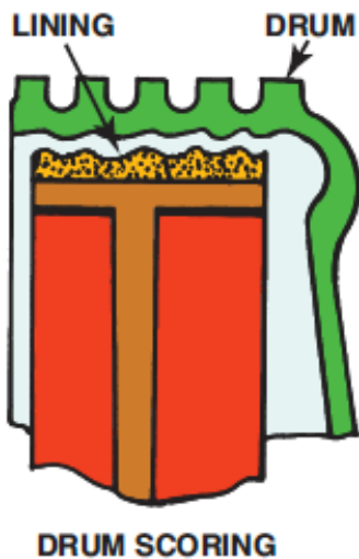
Figure 9. The drum should be machined or replaced.
