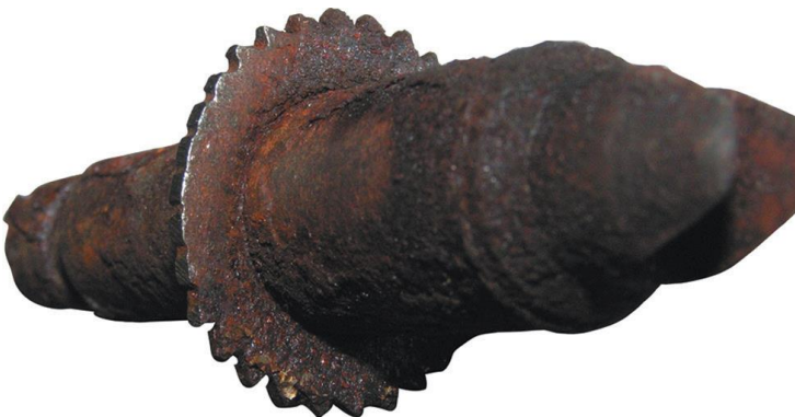
Figure 20. A worn out adjuster starwheel.
