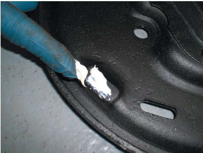
Figure 21. Lubricate the backing plate.
