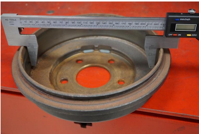
Figure 13. Accurate measurements are made with a brake drum micrometer.
