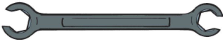
Figure 10. Whenever disconnecting or tightening a brake line, always use the correct size flare-nut wrench.
