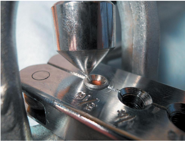
Figure 18. Double flare using the flaring tool.
