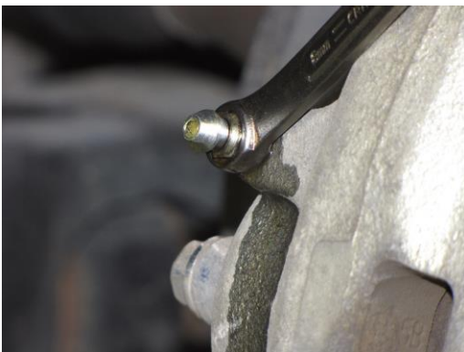
Figure 28. Gravity bleeding is simply opening the bleeder valve and allowing gravity to force the brake fluid out of the bleeder valve.
