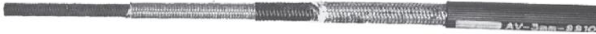
Figure 13. A brake hose is made from several layers of braided and molded material.
