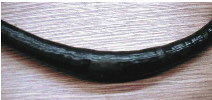
Figure 43. A parking brake cable with internal rust, seizing the cable.
