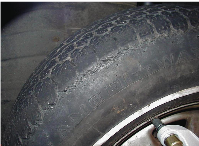
Figure 5. Wear on the outside shoulder only is an indication of an alignment problem.
