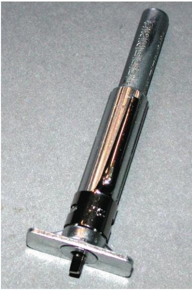
Figure 6. Tread depth gauge.
