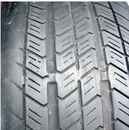
Figure 2. Tire wear indicators.
