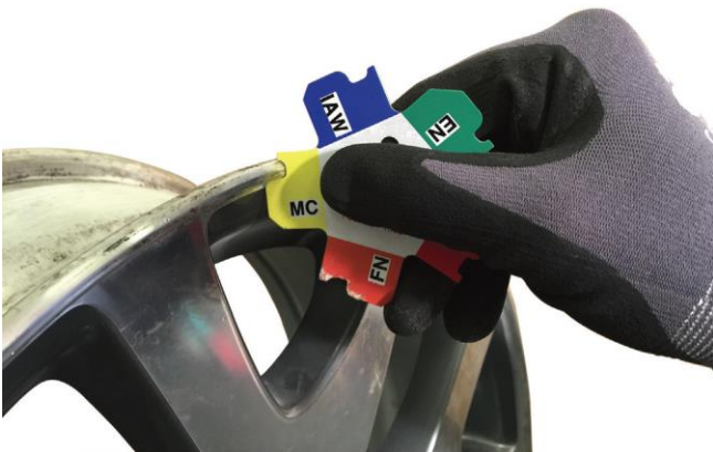
Figure 22. A rim contour gauge is used to select the correct weight type.
