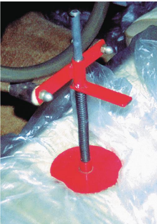
Figure 15. Before adjusting toe, the steering wheel is centered and leveled, then locked in place.
