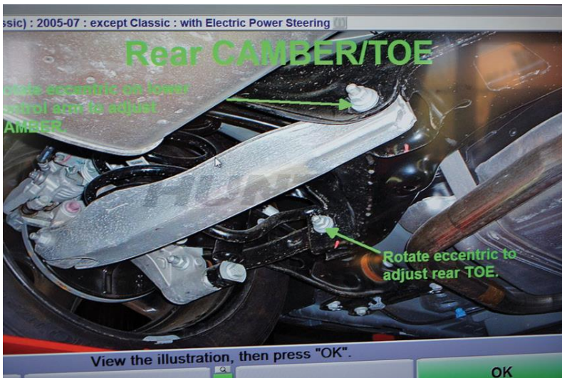
Figure 21. Rear toe adjustment.
