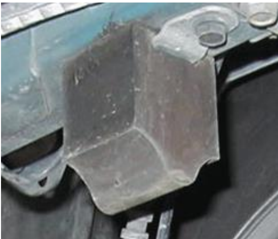
Figure 47. Remove the bolts to replace the bump stop.
