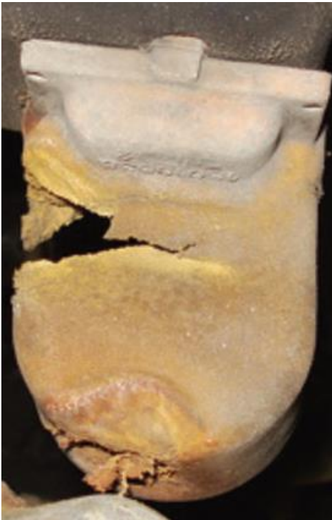
Figure 7. Bump stop damaged by a worn out shock absorber.
