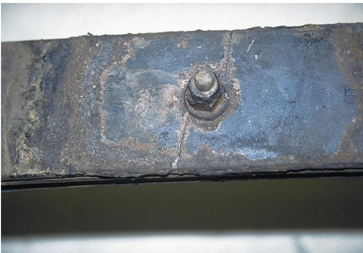
Figure 45. The crack shown is what a technician discovered when the leaf spring was removed during the diagnosis of a sagging rear suspension.
