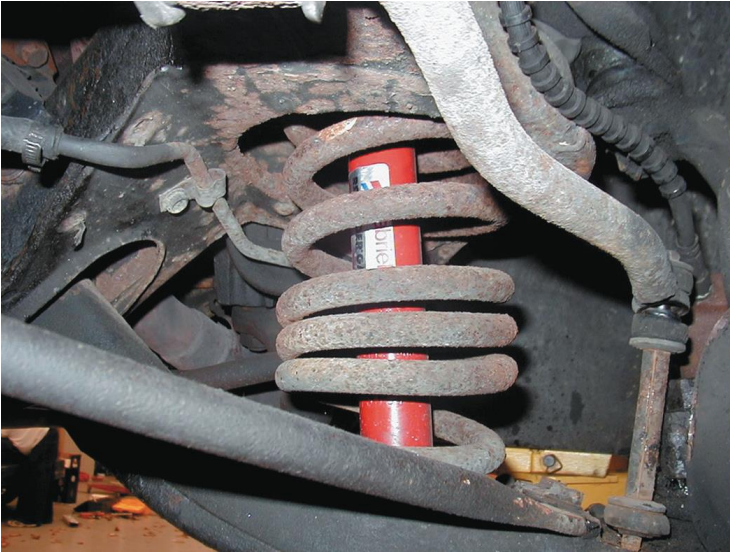
Figure 17. A collapsed front coil spring.
