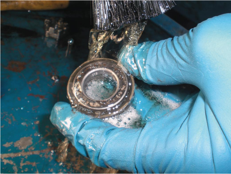
Figure 30. Cleaning the wheel bearing.
