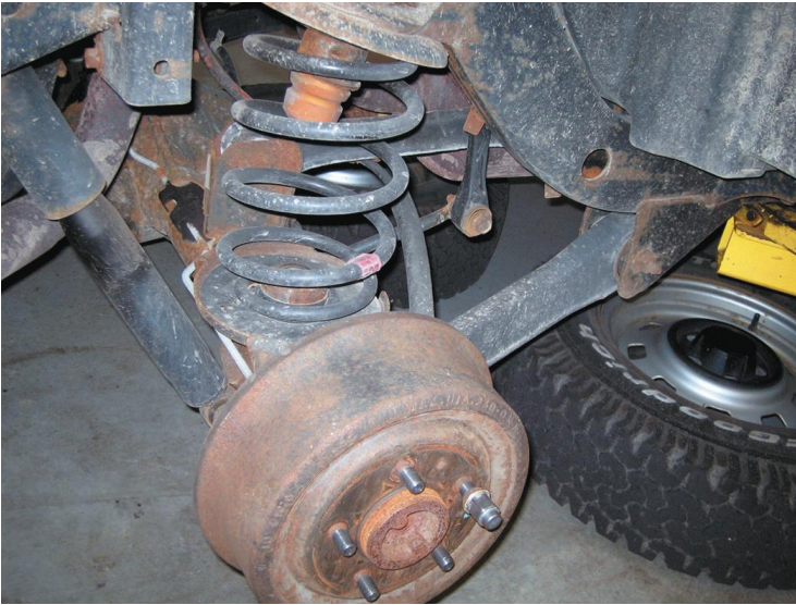
Figure 42. The shock absorber needs to be disconnected before removing the coil spring. Installation is the reverse of the removal procedure.
