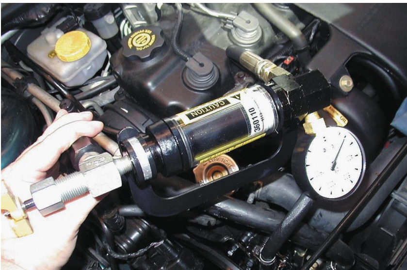
Figure 23. A power steering analyzer that measures both pressure and volume. The shut-off valve is used to test the maximum pressure of the pump.
