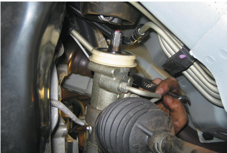
Figure 28. After disconnecting the steering shaft from the rack input shaft, disconnect the power steering lines.
