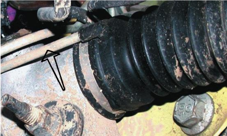
Figure 36. Air bleeder tube, usually on power assisted rack and pinion gears.
