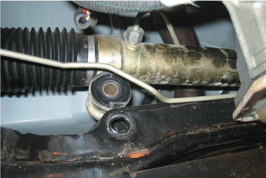
Figure 29. Lower the engine cradle and remove the rack mounting bolts.
