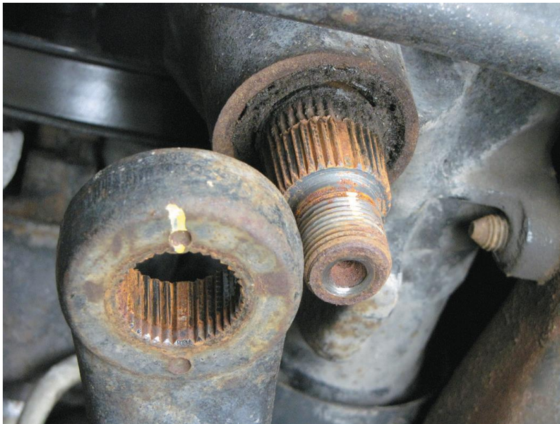
Figure 43. Align the wide index splines when installing the pitman arm.
