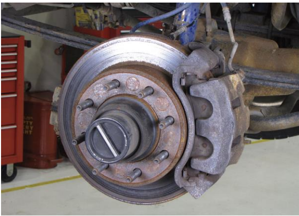
Figure 14. A vacuum operated locking hub.
