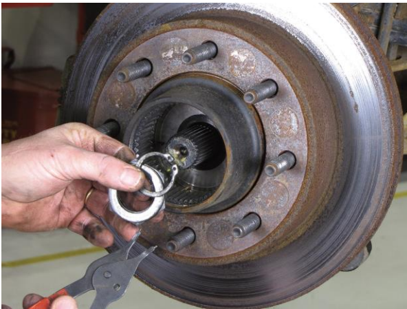
Figure 15. Removing the outer cover and inner snap ring and washer.
