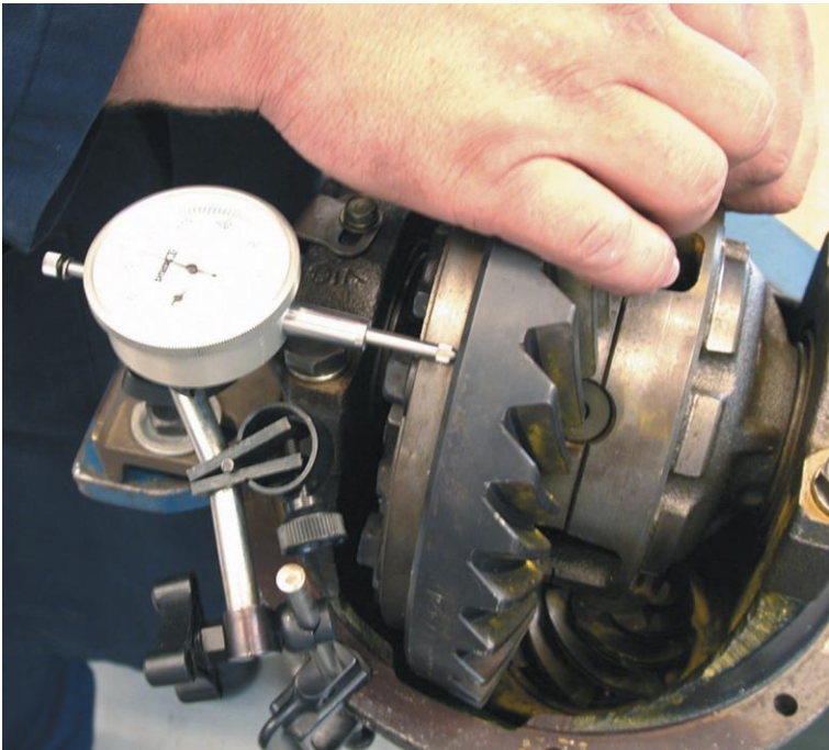
Figure 13. Ring gear runout should be less than 0.002 inch (0.05 mm) as measured by a dial indicator.
