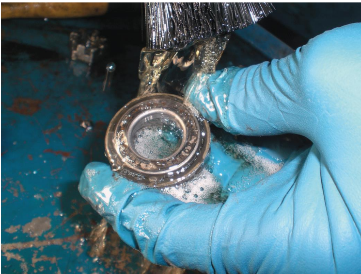
Figure 18. Cleaning the wheel bearing.
