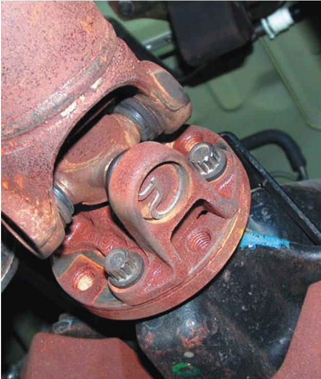
Figure 8. Outside retaining snap ring.
