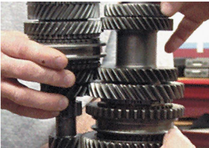
Figure 15. The input shaft (left) and the output shaft (right) are checked for proper assembly before being installed into the case.
