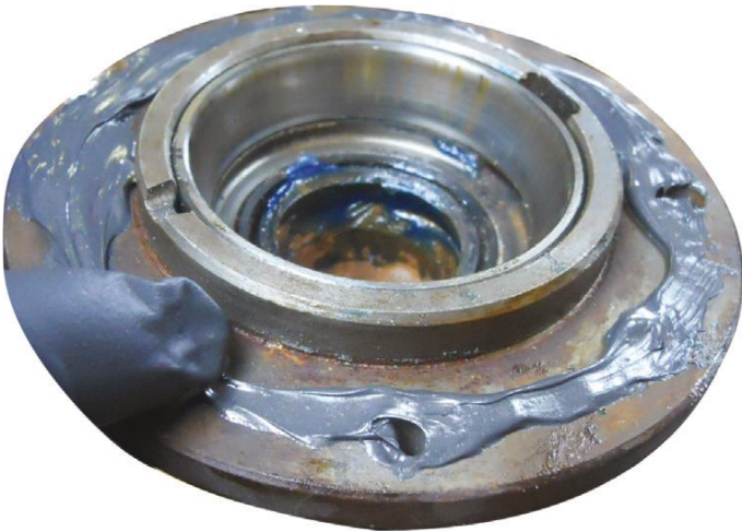
Figure 7. Sealant take the place of a gasket.
