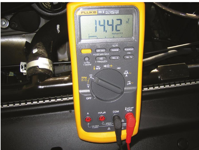
Figure 21. A digital voltmeter measuring battery voltage.
