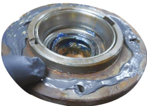
Figure 6. Sealant take the place of a gasket.
