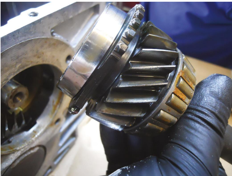
Figure 11. Input shaft gear and bearing.
