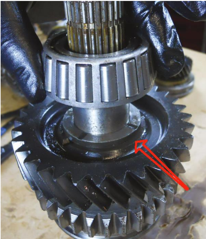
Figure 13. After the bearing is pressed off measure the thrust washer clearance.
