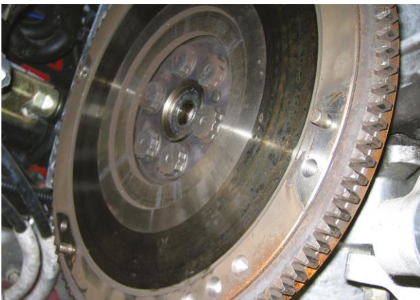
Figure 11. Inspect the ring gear teeth.
