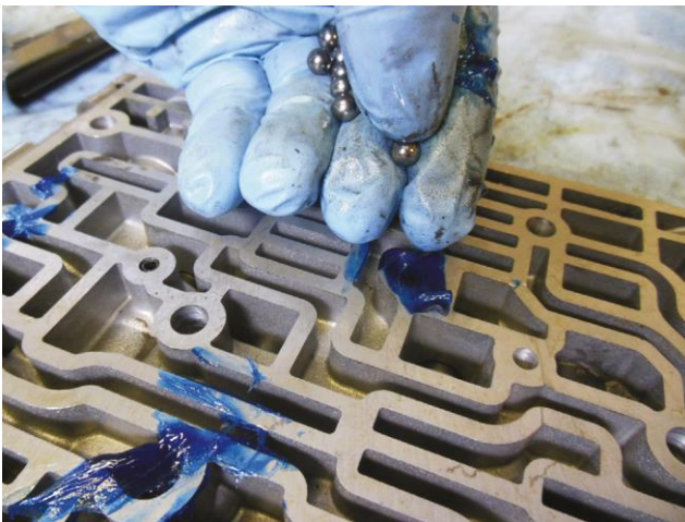
Figure 23. Use assembly lube to keep check balls in position during reassembly.
