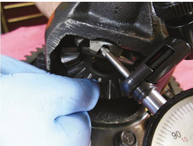
Figure 25. Checking differential gear free play.
