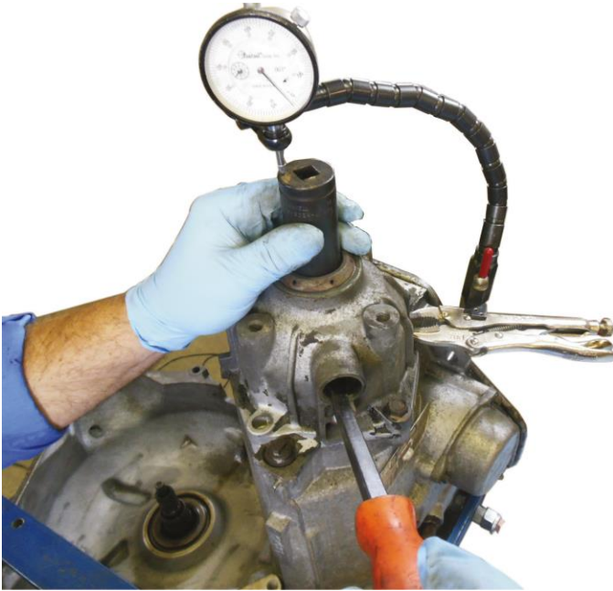
Figure 26. Measuring final drive end play.
