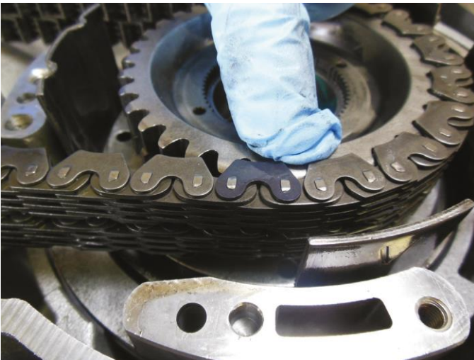
Figure 10. The master link is facing UP and should be reinstated the same way.
