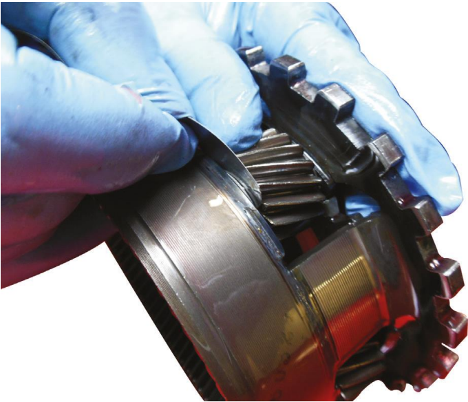
Figure 21. Measuring pinion gear side clearance.
