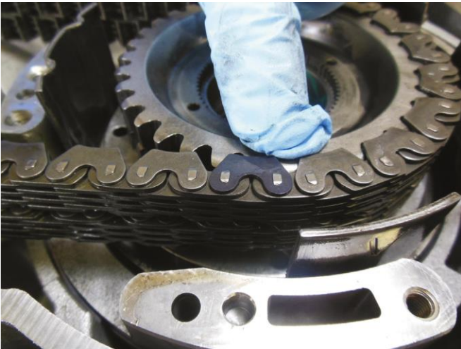
Figure 24. Transaxle drive chain installation.
