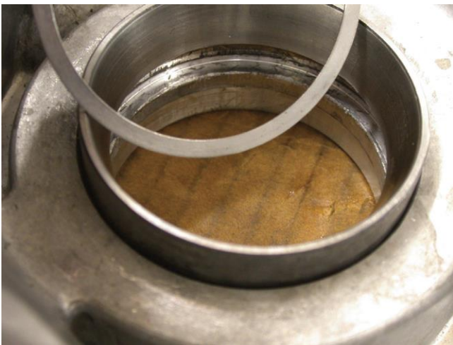
Figure 27. The selective shim is installed behind the bearing cup to give the proper bearing preload.
