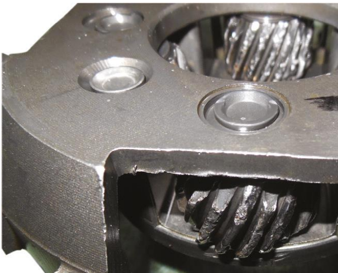
Figure 20. Damaged gear sets are replaced.
