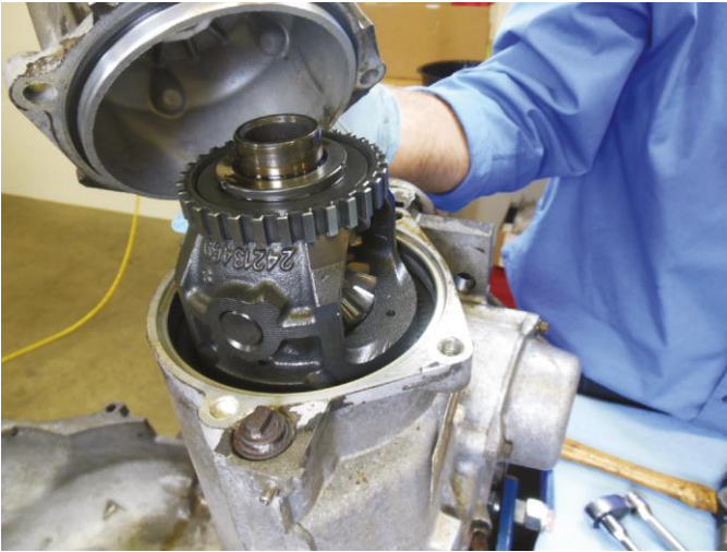
Figure 11. Removing the final drive and differential assembly from a transaxle.
