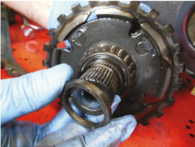
Figure 17. Tapered roller bearing and adjusting shim.
