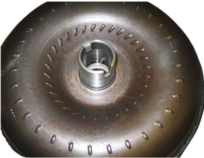
Figure 5. Notches in the converter hub must be aligned with the pump drive tangs.
