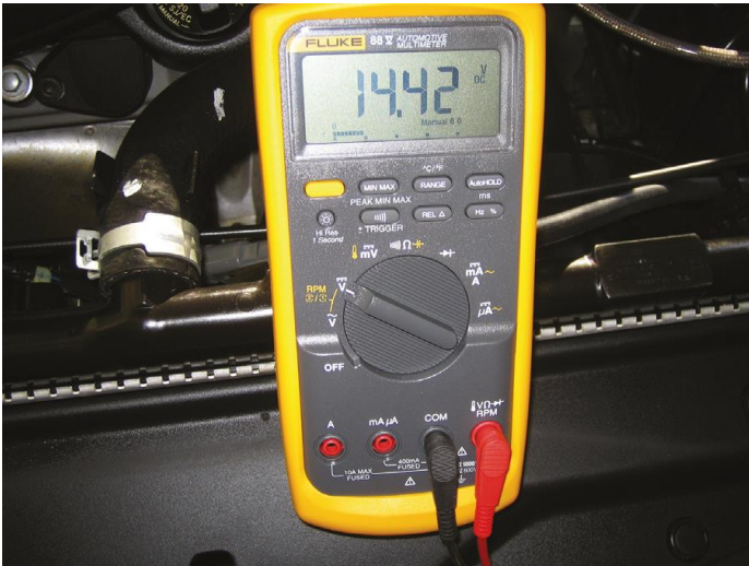
Figure 12. A digital voltmeter measuring battery voltage.
