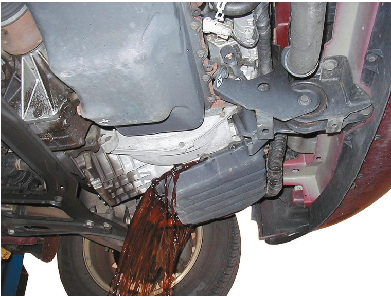
Figure 17. Drain the fluid. Some vehicles have a transmission drain plug.
