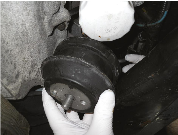
Figure 16. Replacing a power train mount.
