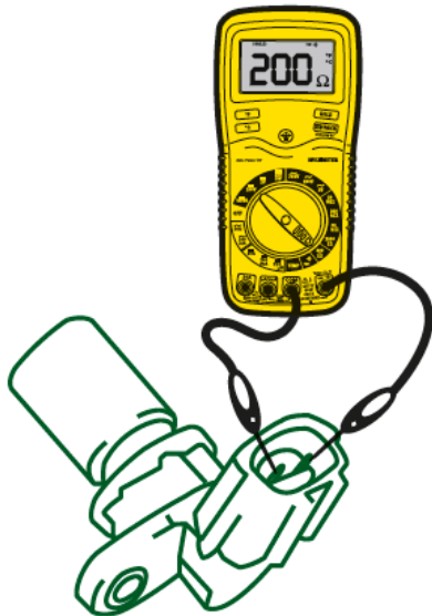
Figure 17. Measuring CKP sensor resistance.
