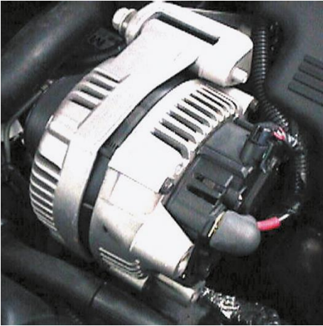
Figure 10. Alternator (also called a generator).
