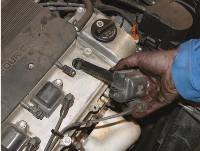
Figure 16. Check the COP coil for arcing or corrosion.
