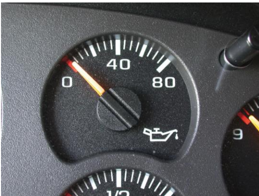
Figure 2. The dash oil pressure gauge may be a good indicator of engine oil pressure. If there is any concern about the oil pressure, always use a mechanical gauge to be sure.
