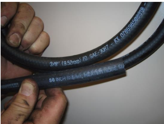
Figure 16. The top 3/8 inch hose is designed for oil and similar liquids, whereas the 3/8 inch hose below is labeled “heater hose” and is designed for coolant.
