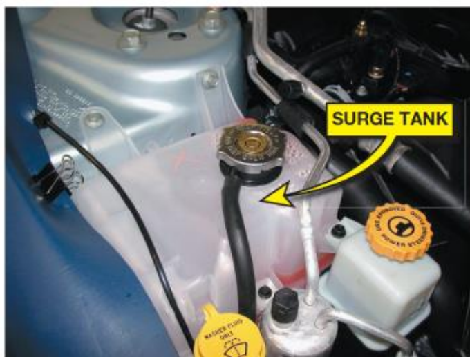
Figure 14. Surge tank and pressure cap.
