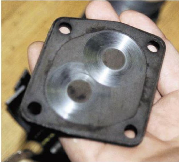
Figure 6. A worn oil pump end plate.
