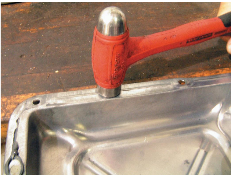
Figure 40. Straightening an oil pan.
