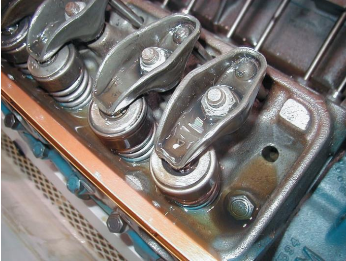
Figure 41. The engine should be pre-lubed until oil is seen.
