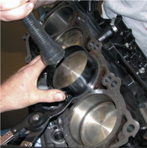
Figure 31. Installing the piston.
