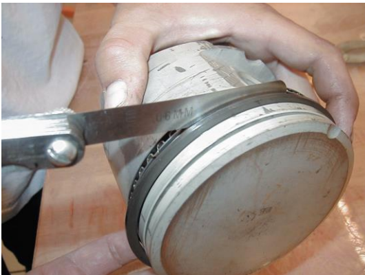
Figure 28. Checking piston ring side clearance.
