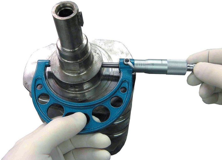
Figure 16. Measuring a crankshaft main journal.
