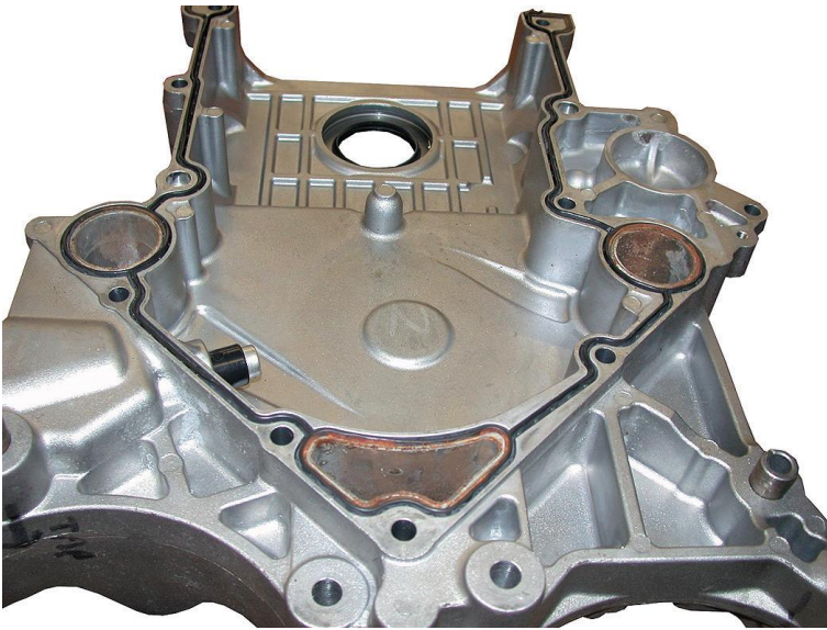
Figure 35. A front engine cover sealed with a formed in place gasket.
