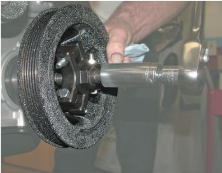
Figure 8. Removing the vibration damper.
