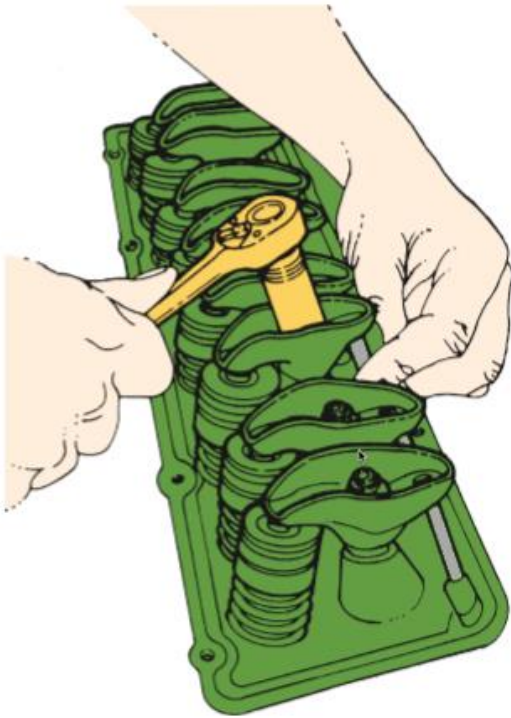
Figure 20. Adjusting to zero lash.
