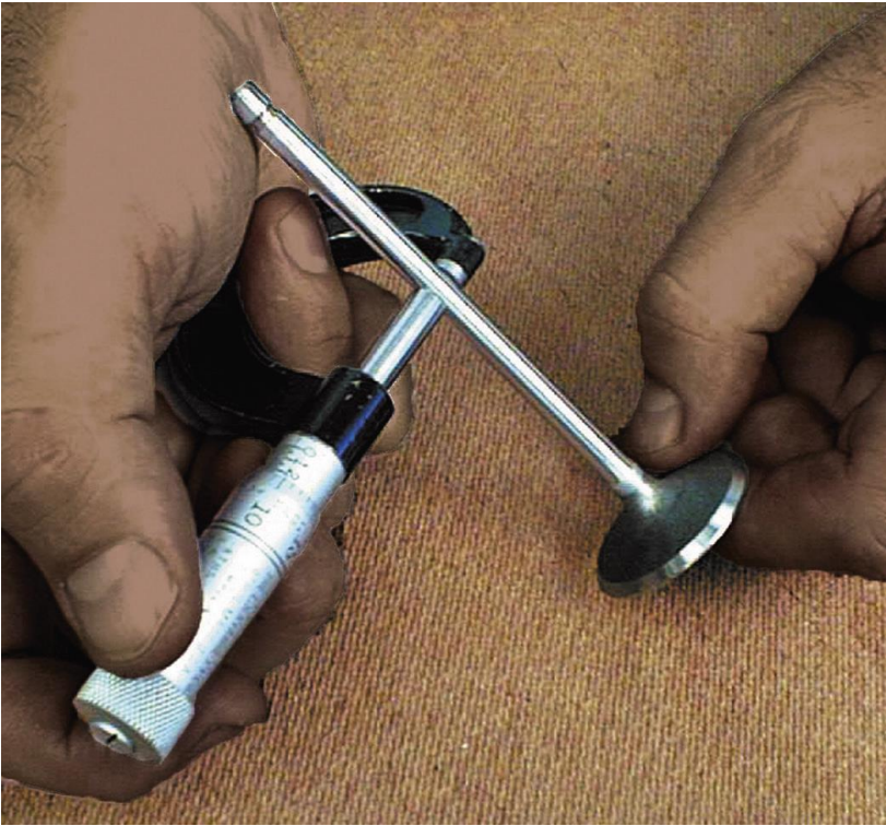
Figure 13. Measuring valve guide and valve stem using a micrometer.
