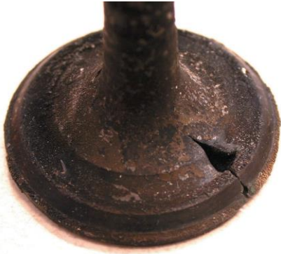
Figure 9. A valve damaged by excessive temperature in the combustion chamber.
