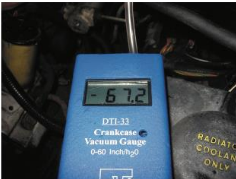
Figure 11. This gauge measures vacuum in units of inches of water to test the vacuum at the dipstick tube. Note that 28 inches of water equals 1 psi, or about 2 inches of mercury (inch Hg) of vacuum.
