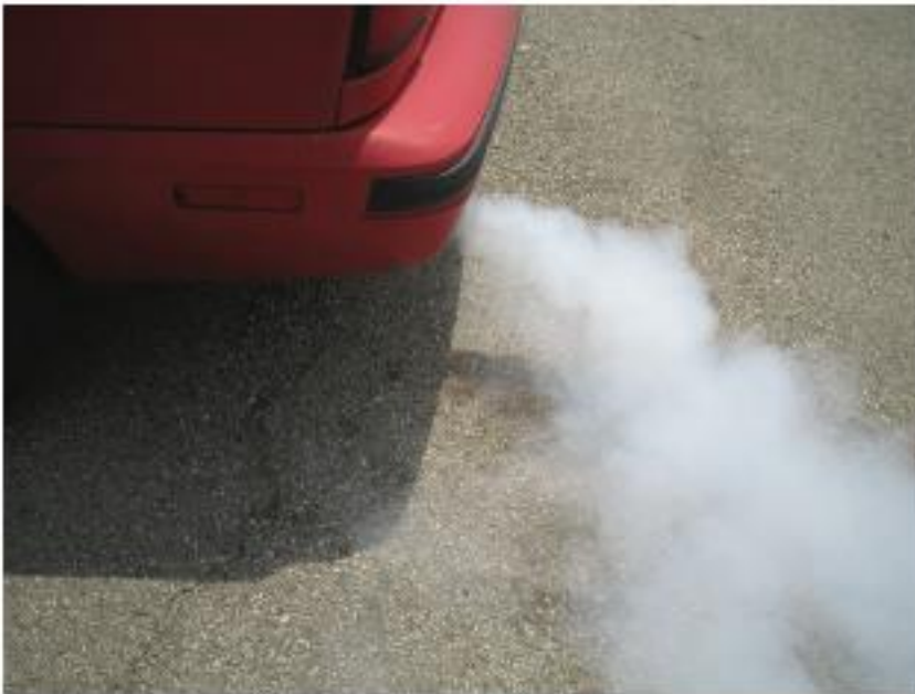
Figure 8. Excessive white exhaust indicates water or coolant in the combustion chamber.
