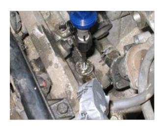
5. Reinstall the EGR valve with a new gasket and check the engine for proper operation.
