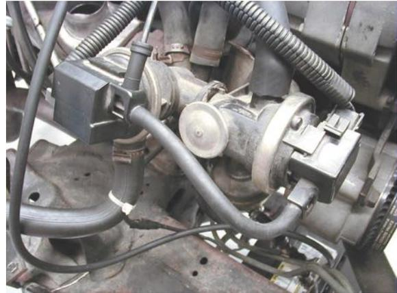
\_\_\_\_\_ 3. Start the engine and feel the air pump lines to confirm the proper air flow.
