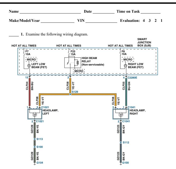
2. The vehicle problem is that the left headlamp does not light on high or low beam. The right headlamp lights normally. Use the diagram to identify where the fault could be.
