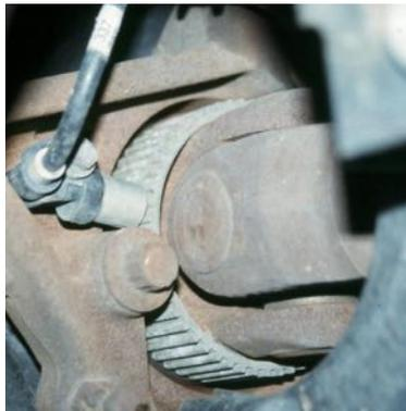
\_\_\_\_\_ 4. With the meter still set to read ohms, connect one meter lead to a good clean chassis ground and the other lead to one terminal of the WSS connector. This test determines that the WSS is shorted to ground unless the meter indicates infinity (OL).
