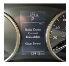
radar cruise control. In automated vehicles, the sensors need to be heated, and maybe cleaned, so that they can operate under all driving conditions.
