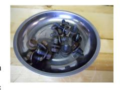
trays are an excellent tool to help keep fasteners organized so they do not get misplaced. Some technicians use a separate tray for the fasteners from each major component such as the valve body bolts.
