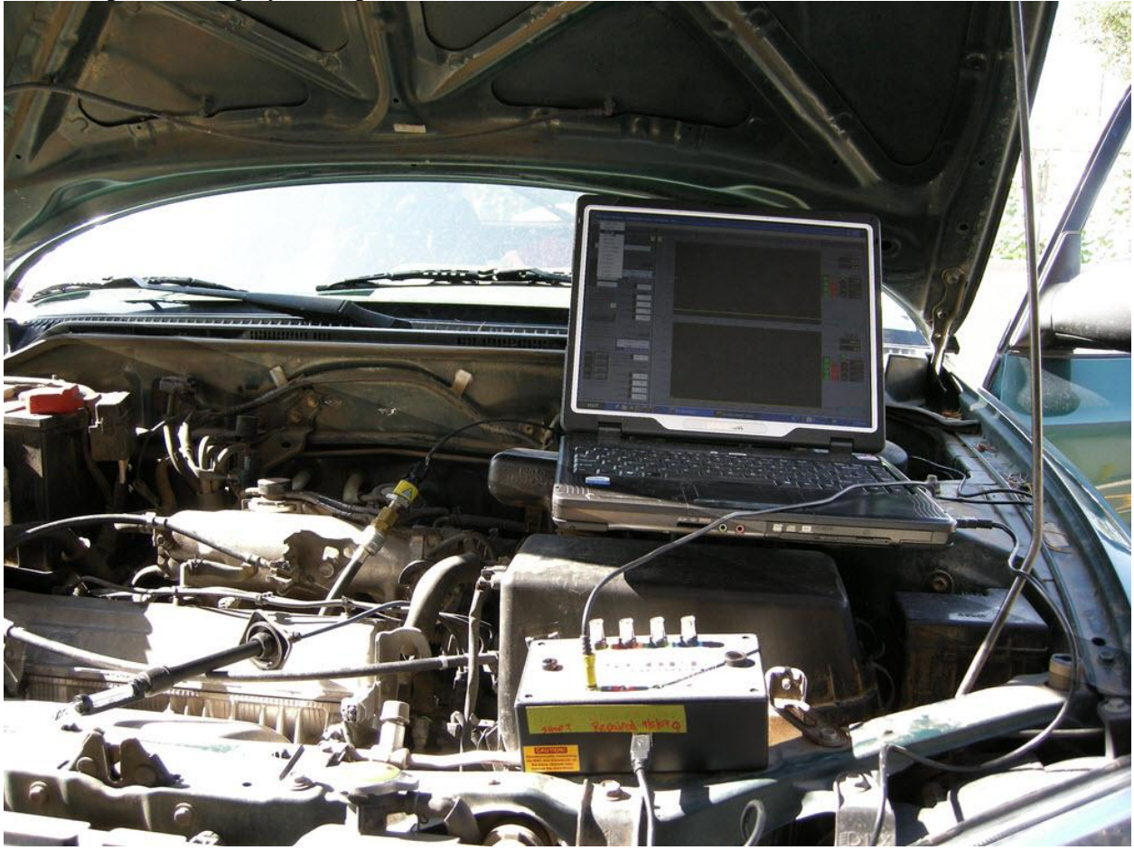
Test setup for testing cylinder pressure.
