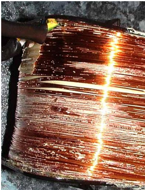
Solenoid coil with the case removed.
