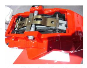
technicians are simply replacing the old used calipers with "loaded calipers." Loaded calipers are remanufactured calipers that include (come loaded with) the correct replacement friction pads and all the necessary hardware. Therefore, only one part number is needed for each side of the vehicle for a complete disc brake overhaul.
