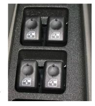
and holding the down button for 10 seconds. If the vehicle is equipped with an auto up feature, repeat the procedure by holding the button up for 10 seconds. Always check exact service information for the vehicle being serviced.
