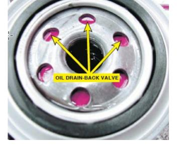
rather than having no lubrication, if the filter becomes plugged. The oil also goes through the bypass when the oil is cold and thick.
