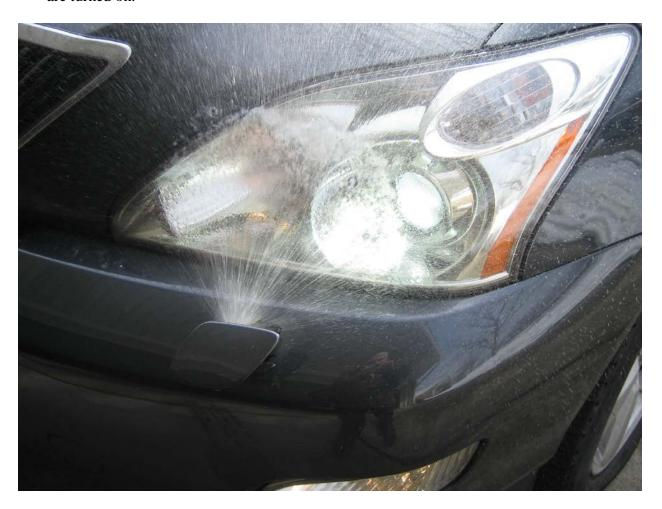
**Caption:** Headlight washers usually only work when both the headlights and the wipers are on. When the windshield washers are activated, the headlight washers spray, but usually only once per ignition key cycle.
