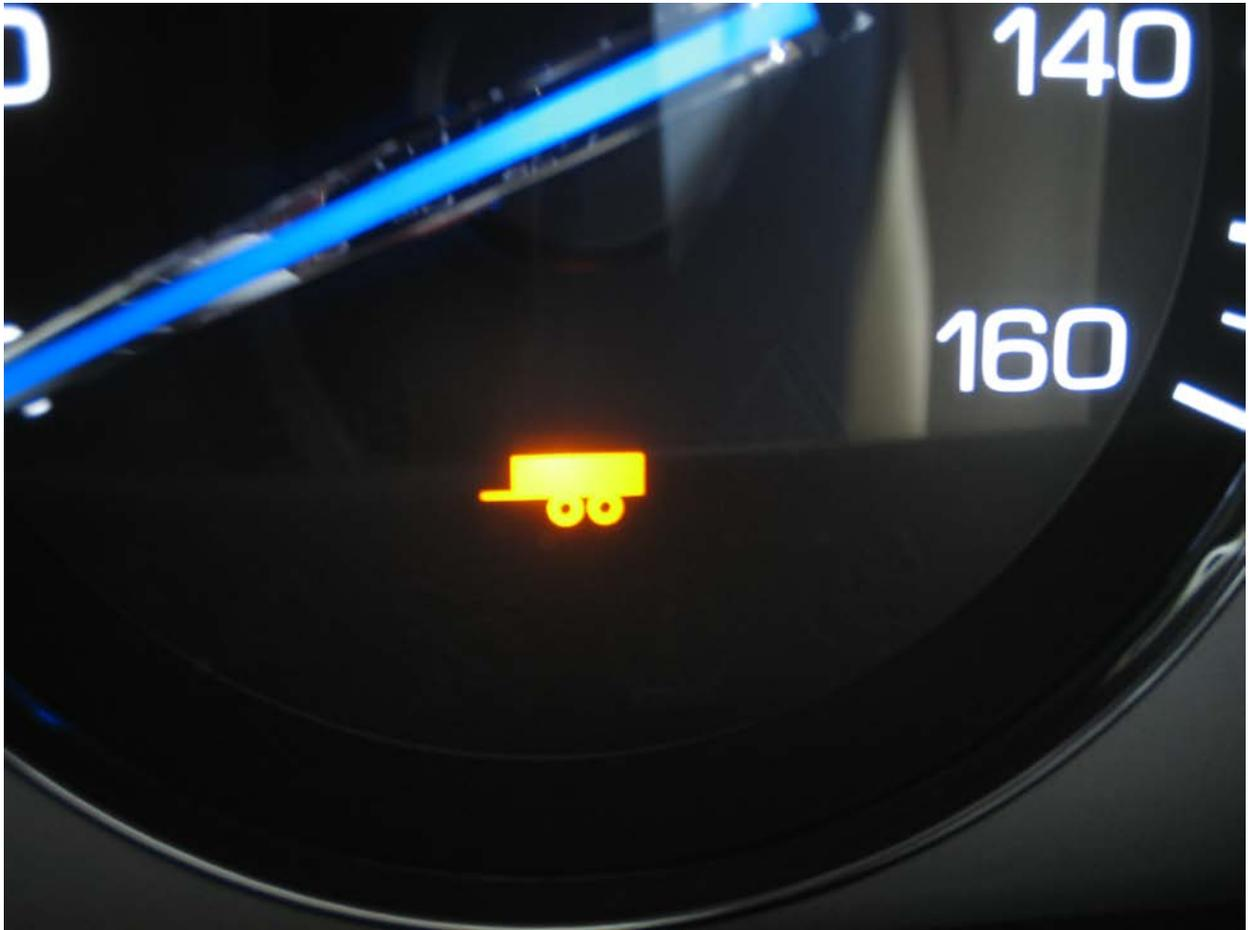
**Caption:** A trailer towing icon on the dash indicates the driver has selected the trailer towing mode.
