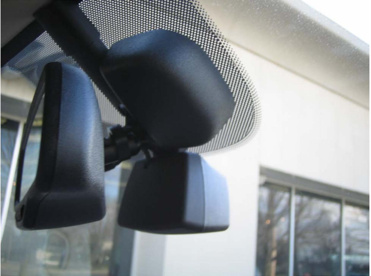
**Caption:** The forward-facing camera (below the rain sensor) is used to control high-beam headlights.
