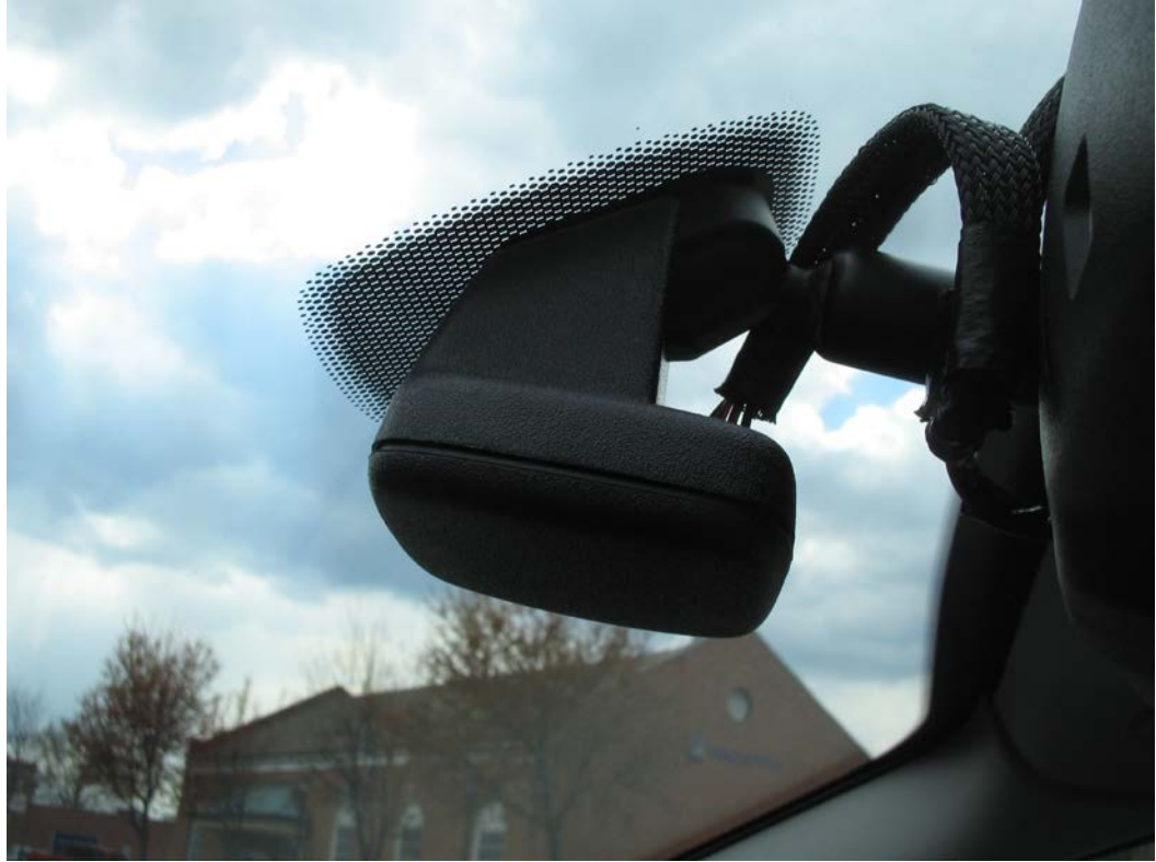
Caption: The view of a headlight camera on this Cadillac pointing forward can detect headlights coming toward the vehicle so that the controller can select low-beam headlights. (Photo by James Halderman)
