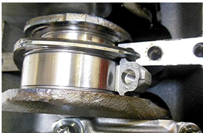
\_\_\_\_\_ 3. Measure the crankshaft journals and compare to specifications.
