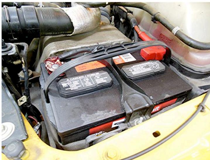
\_\_\_\_\_ 2. Perform a key-off battery drain (parasitic load) test. Battery drain = \_\_\_\_\_.
