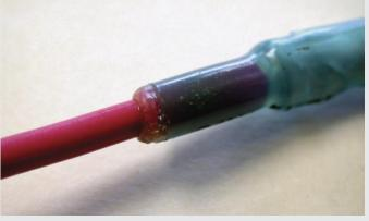
tubing. This method is recommended by Chrysler and it uses the special heat shrink that has glue inside that melts when heated to form a sealed connection. Regular heat shrink tubing can be used inside a vehicle, but should not be used where it can be exposed to the elements.
